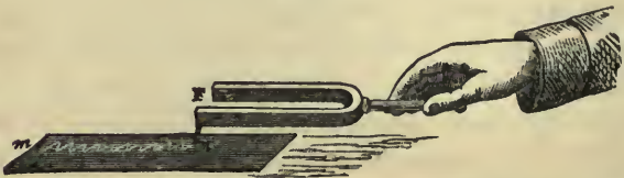
FIG. 36 (Tyndall). Illustrates how the vibrations of a tuning-fork are registered on a blackened (smoked) glass. In order that the movements of the fork shall be traced in the form of regular curves, the surface must be kept moving at a definite regular rate.
